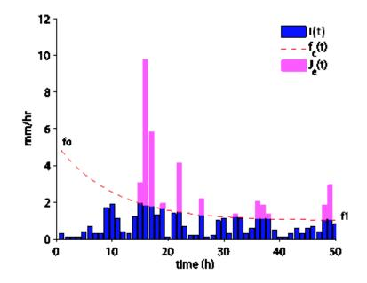
Figure 2: Infiltration rate with initial and maximum infiltration capacities
