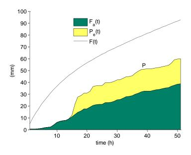
Figure 3: Infiltration components for Horton's method
