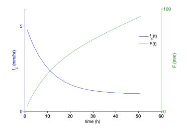
Figure 1: Infiltration capacity and cumulative infiltration
