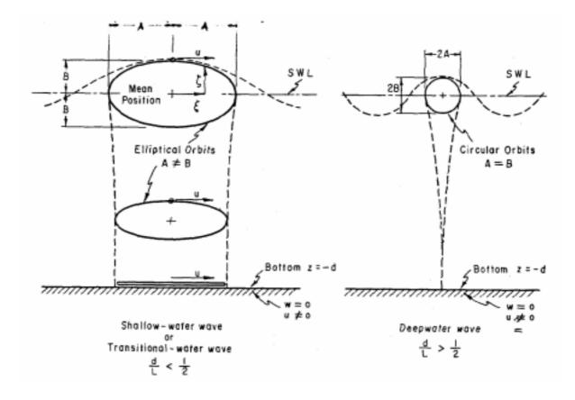
Fig. 6.2: Water particle displacement from the mean location for shallow water and deep water waves. (From the Shore Protection Manual Vol. 1 p. -2-17)
