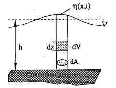
The potential energy contained in a column of water with cross section dA as shown on the graph is
