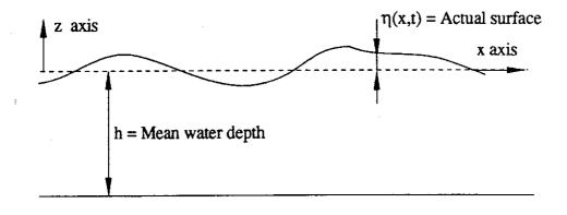
Fig. 3.1: Waves along a channel
