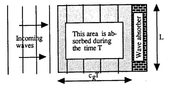
During a time interval *T*, all energy within the dashed area is absorbed by the wave absorber. The energy within the square is
