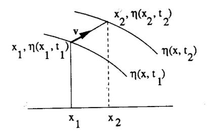
Figure 3.2: Motion of a fluid point on the free surface
