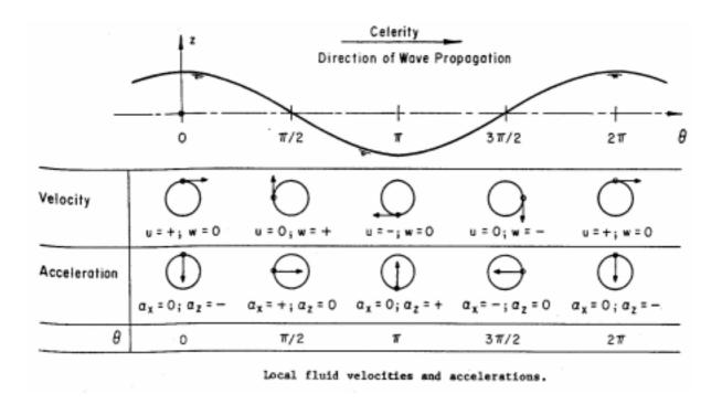
Fig. 6.1: Surface elevation along with velocity and acceleration vectors (From Shore Protection Manual, Vol. 1 p. 2-14)
