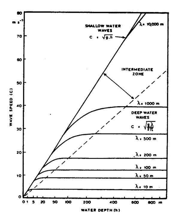
Fig. 5.2: The phase velocity of regular water waves (From Bowden, 1983)
